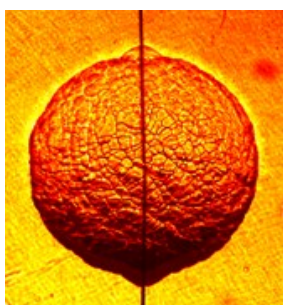
Image II: Laminar, diffusion-thermally unstable, hydrogen-air premixed flame of equivalence ratio: 0.6 at 5atm pressure.
