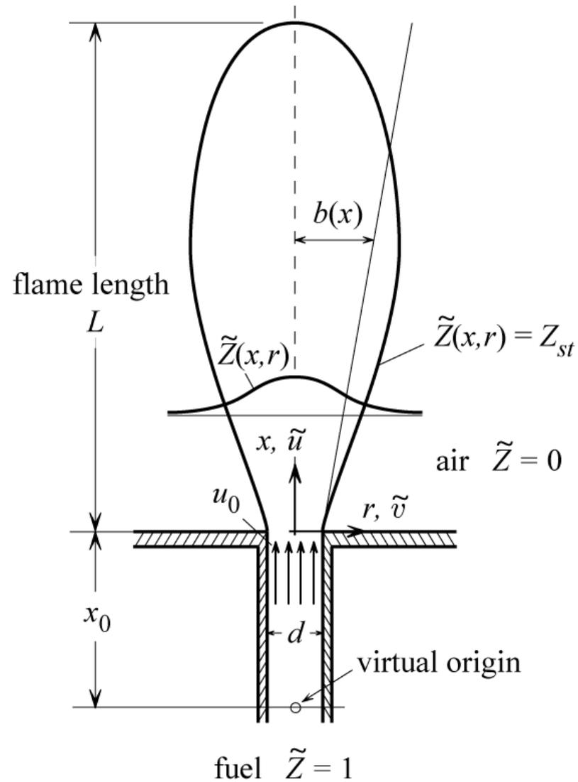
Using Favre averaging and the the boundary layer assumption we obtain a system of two-dimensional axisymmetric equations
