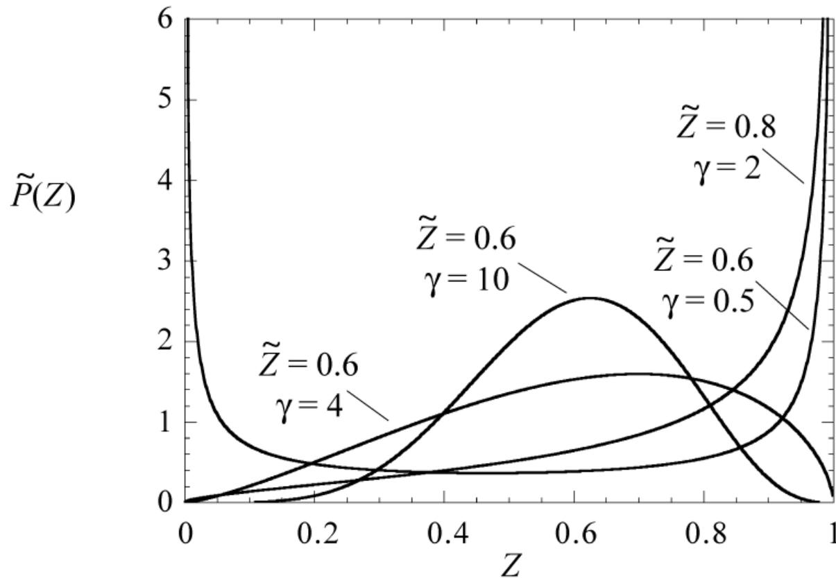
It can be shown that in the limit of very small  $\tilde{Z}''^2$  (large  $\gamma$ ) it approaches a [Gaussian distribution](#).
