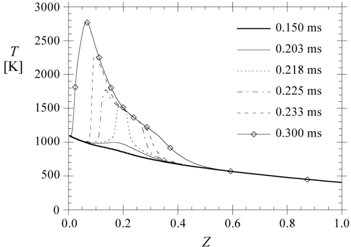
It is seen that auto-ignition starts after 0.203 ms, when the temperature profile shows already a small increase over a broad region around  $Z=0.2$ .
