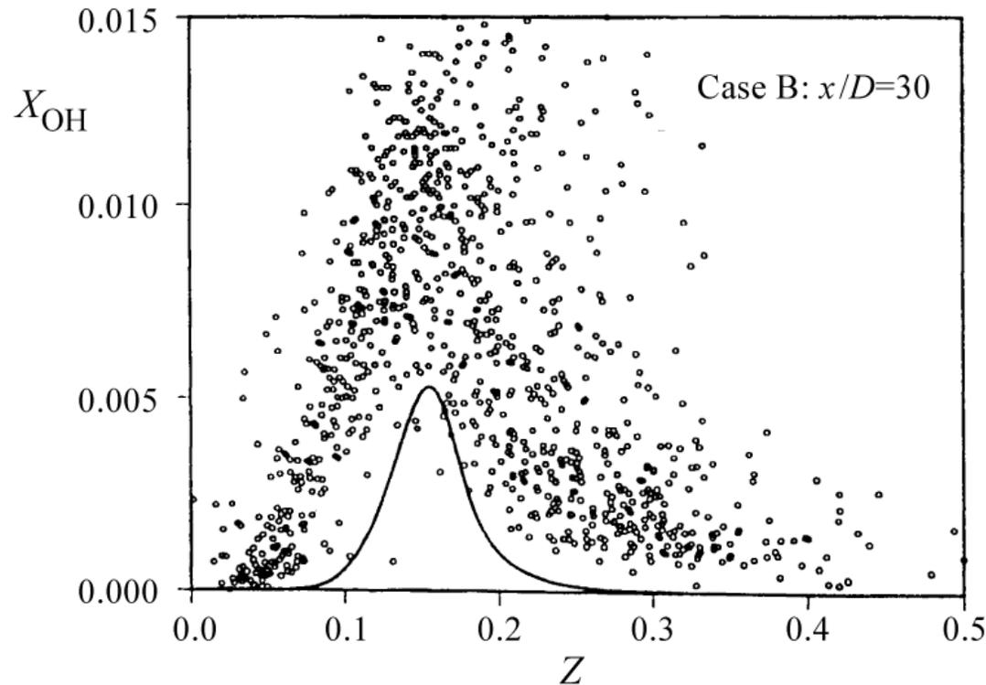
The flamelet calculations show an increase of the maximum values by a factor of 3 already at the low strain rates  $a = 100/\text{s}$  and  $a = 1000/\text{s}$ .
