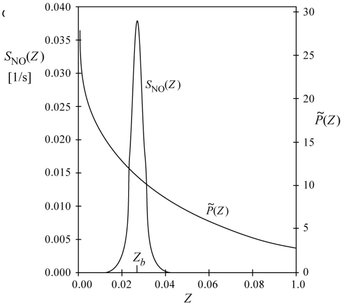
The NO reaction rate acts nearly like a  $\delta$ -function underneath the integral in
