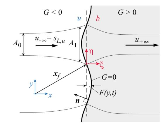
Gas expansion in the flame front lead to a deflection of a stream line that enters the front with an angle.
