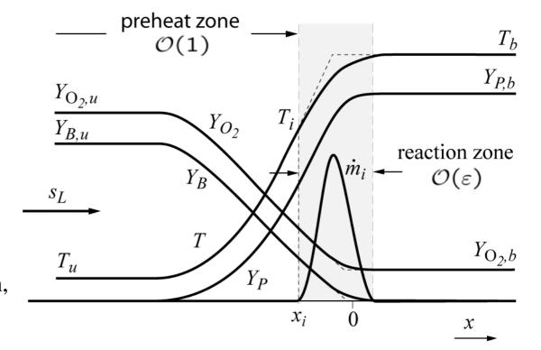
Heat conduction from the reaction zone is also directed upstream leading to a preheating of the fuel/air mixture. Therefore the region upstream of the reaction zone is called the preheat zone.
