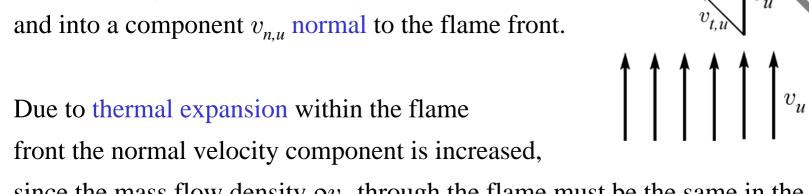
since the mass flow density  $\rho v_n$  through the flame must be the same in the unburnt mixture and in the burnt gas (subscript b).
