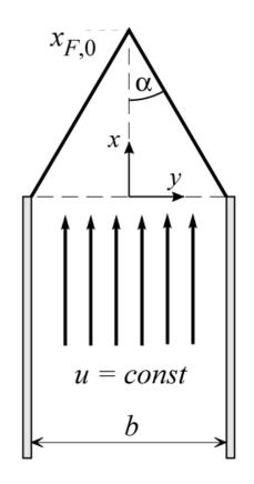
which is equivalent to  $s_{L,u} = v_{n,u} = v_u \sin \alpha$ .
