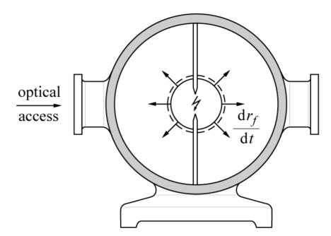
At the flame front the kinematic balance between propagation velocity, flow velocity and burning velocity with respect to the unburnt mixture is
