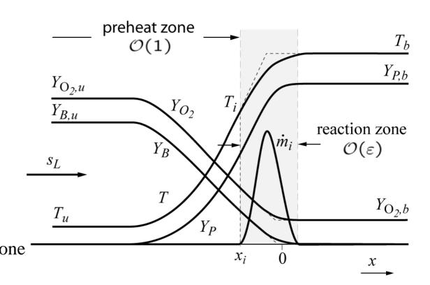
The fuel is entirely depleted while the remaining oxygen is convected downstream where it has the mass fraction  $Y_{O_{2,u}}$ .
