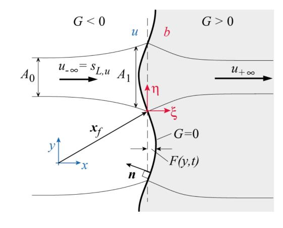
At a cross section  $A_1$ , where the density is still equal to  $\rho_u$  the flow velocity due to continuity and the widening of the stream tube is
