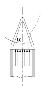
Explanation: the strong curvature of the flame front at the tip leads to a preheating by the lateral parts of the flame front and thereby to an increase in burning velocity.
