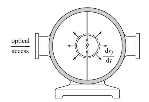
Spherical propagation of a flame then takes place which may optically be detected through quartz windows and the flame propagation velocity  $\mathrm{d}r_f/\mathrm{d}t$  may be recorded.
