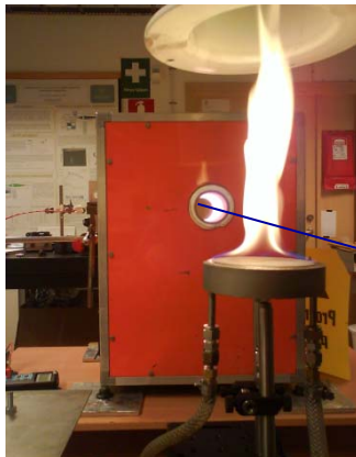
LIDAR measurement, Oven, 300 acquisitions Rayleigh Temperatures
