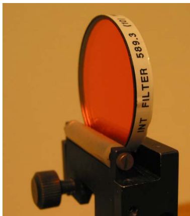
Interference filter with centre wavelength of 589.3 nm and with FWHM of 10 nm.
