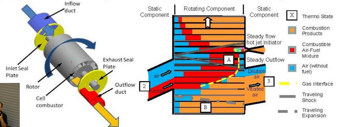
*The channels in the sketch at the right represent the tubes in the rotor at the left - but “unwrapped” at a moment in time. The rotor revolution is driven by a motor at a speed selected to allow the flame to complete the channel combustion within a rotation.*
