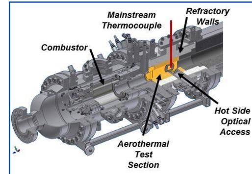
*Test rig for advanced aerothermal cooling development*
