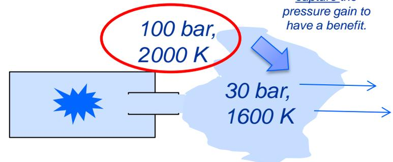
Pressure -gain combustion
