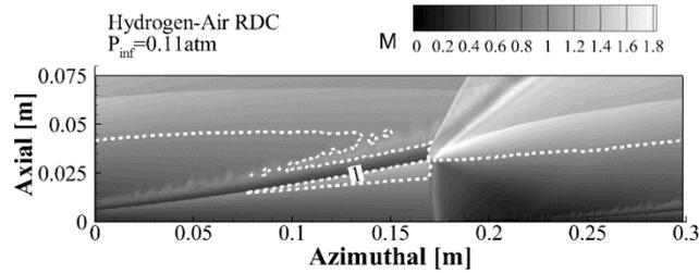
*Mach number contours for  $P_{out}=0.11\text{atm}$  (top) and  $P_{out}=2\text{atm}$  (bottom)*
