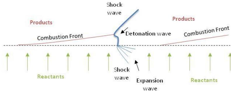
Combustion annulus unrolled. Reactant flow from the bottom.
