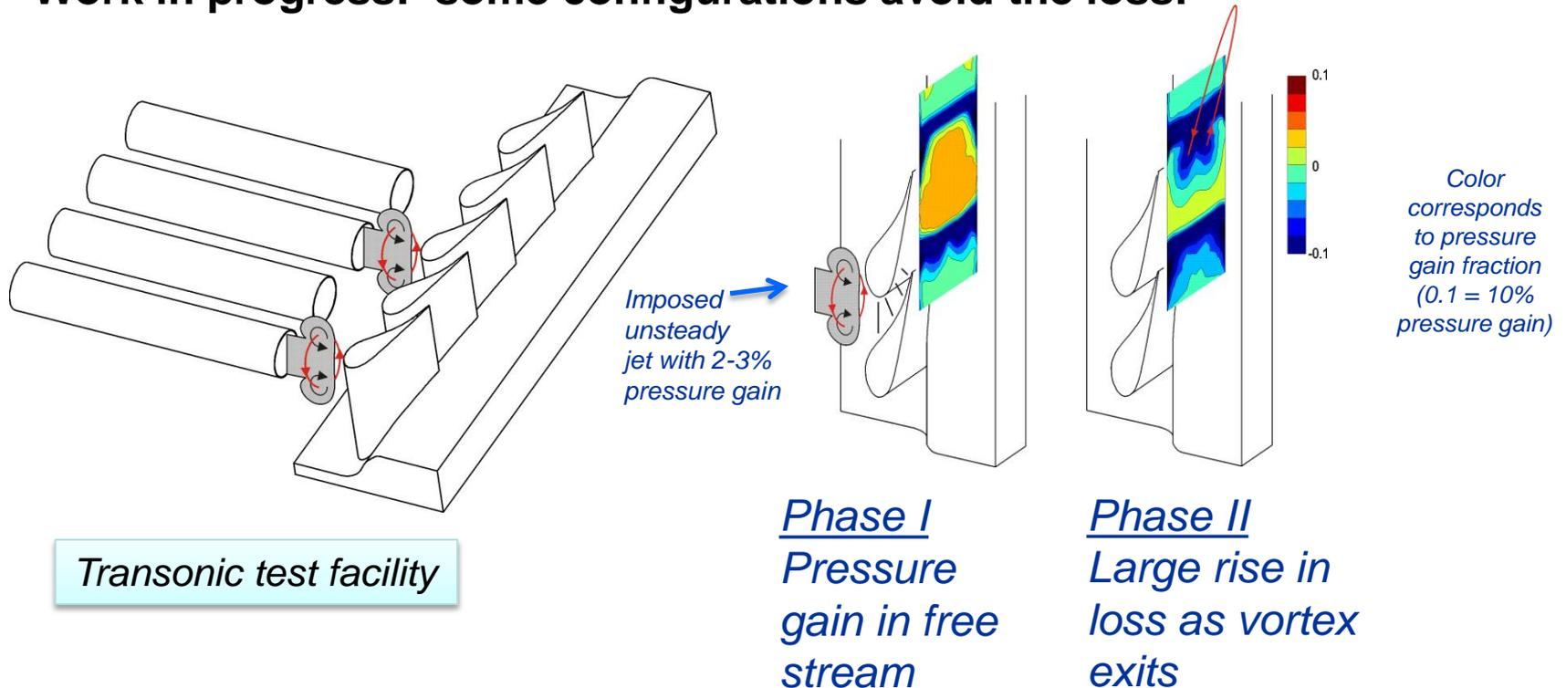
Cause of loss : Vortex interacting with vane suction surface.
