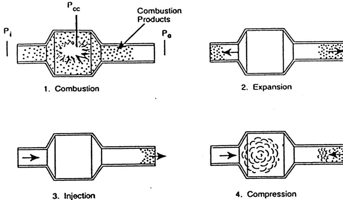
**Fig. 1 Operation of an aerodynamically valved pulse combustor. The combustion event (1) raises the pressure in the combustion chamber ( $P_{cc}$ ), forcing gas out of the inlet pipe and tailpipe (2), the momentum of fluid in the tailpipe draws fresh air through the inlet (3), with a subsequent compression of gases in the combustion chamber (4). On a time average, the flow is from left to right.**
