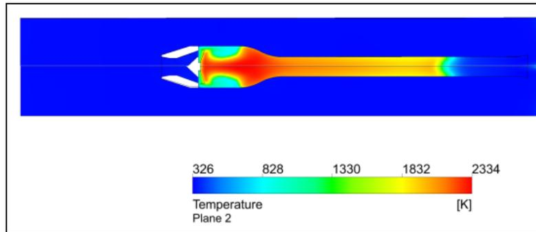
*Simulation of pulse-jet behavior –with NO<sub>x</sub> emissions and experimental validation.*
