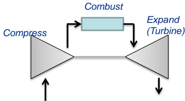
Note that the “gas dynamic engine” does not have constant pressure combustion as in a turbine; the analogy is not perfect!
